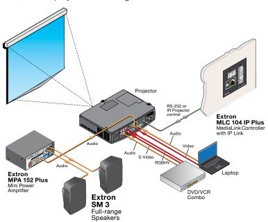
Figure 1. Typical Application for the MPA 152 Plus
